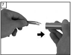
Thread lead wires and safety cable through downrod as shown.
